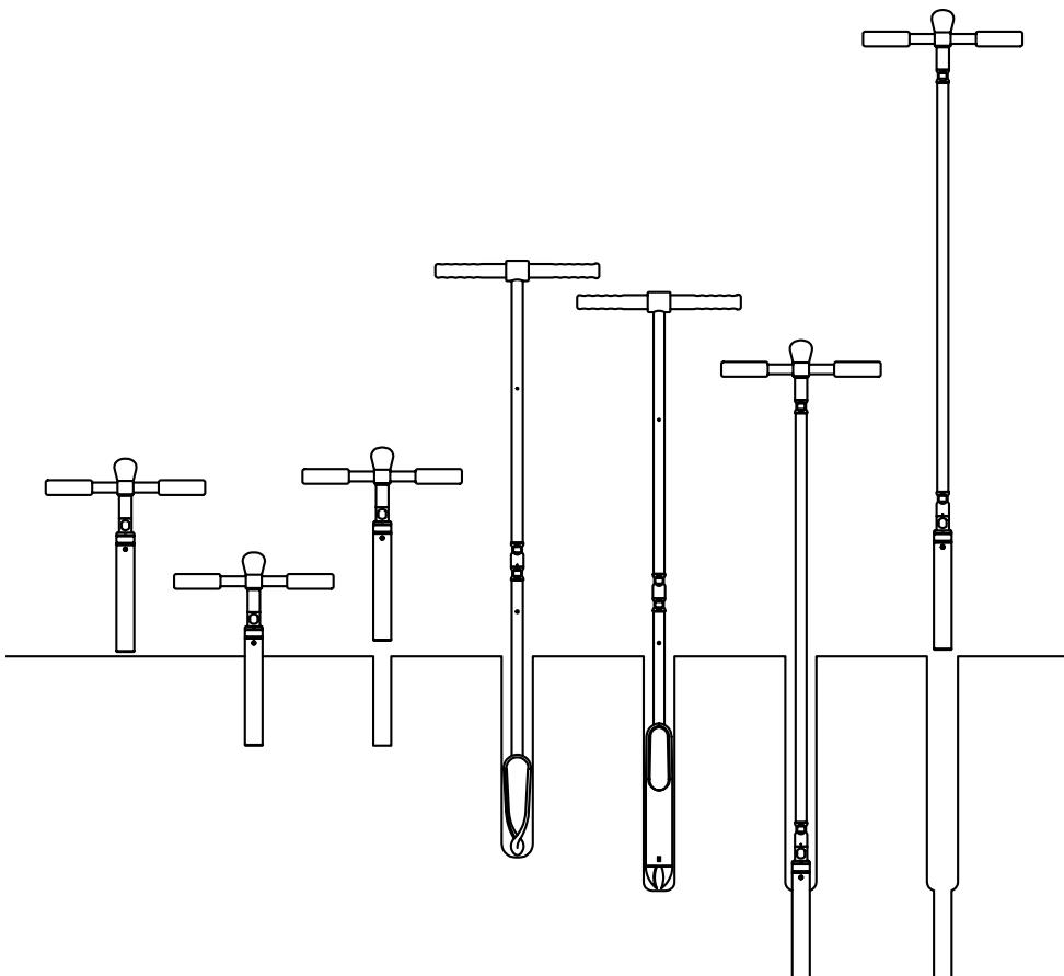
6. Screw and press the auger into the soil. The Riverside auger creates a level horizontal profile. Pull out the auger without rotating it. Tap it gently on the surface and the sample will detach itself.
