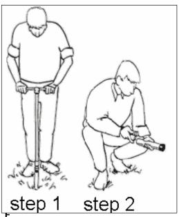
**Figure 4:** Surface sampling. <u>Step 1</u>-Push the core apparatus with sample core in the soil and take the sample from the soil. <u>Step 2</u>-Add the filling blocks in the sample tube and cap the sample tube.
