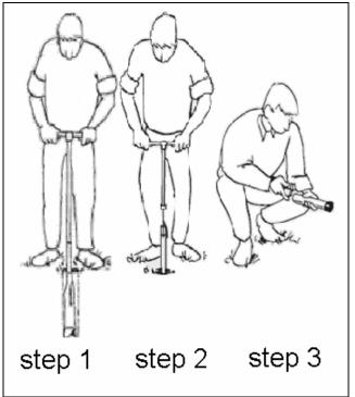
**Figure 5:** Sampling under surface. <u>Step 1:</u> Pre-bore to the required depth with the edelman auger bore. Next the Riverside auger can be used to make the bottom of the hole flat. <u>Step 2:</u> Push the core apparatus with sample core in the soil and take the sample from the soil. <u>Step 3:</u> Add the filling blocks in the sample tube and cap the sample tube.
