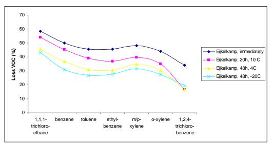
Figure 3. VOC loss for different Eijkelkamp methods.
