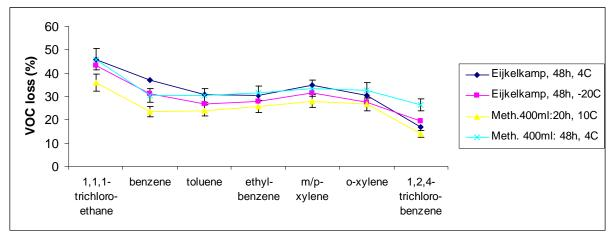
Figure 5. VOC loss (%) for Eijkelkamp method (48h, 4°C; 48h, -20°C) compared with 400ml methanol method (20h, 10°C; 48h, 4°C).
