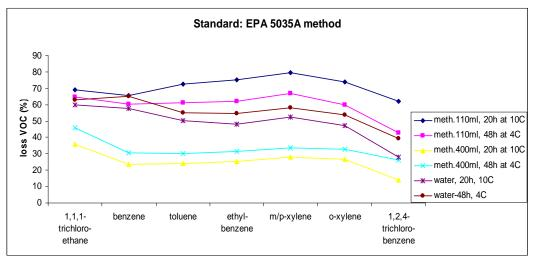
Figure 4. VOC loss for the three standard methods (with water or methanol)
