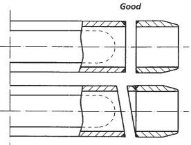
Ensure that this is done as straight as possible (the two parts should preferably turn flush up against each other) to avoid problems when welding on the new cutting shoe.
