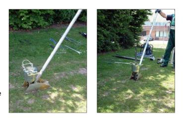
Avoid knocking sand and stones into the borehole when raising the gouge.
