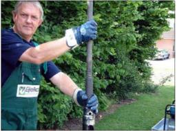
Place the gouge with the extension rod into the borehole.
