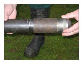
Attach a coupling sleeve and striking pen to the core sampler, place the percussion hammer and hammer the core sampler into the ground. Withdrawing it from the ground is effected as described for the percussion gouges (see page 5).
