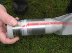
Take the extension pipe and slide the foil guide cylinder with foil and foil ring into the extension pipe.
