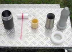
Take the thin-walled PE foil, unroll the first 20 cm and slide this over the stand to the end of the foil guide cylinder. Slide the rest of the foil over the guide cylinder.
