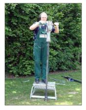
Hammer the percussion gouge into the ground. Remove the percussion hammer. Unscrew the striking pen from the coupling sleeve. If this is stuck, unscrew it using the tools supplied.
