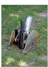
Place the universal casing and rod puller clamp on the mechanical rod puller and then place the clamping jaw in the casing and rod puller clamp. Check whether the filling ring has been fitted.
