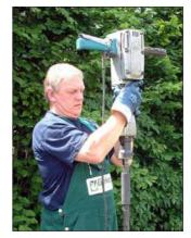
Stand on the step-up. Start the percussion hammer and keep the machine as upright as possible during hammering. If the percussion gouge "finds its own way", follow this direction with the machine. Do not force it to one side.
