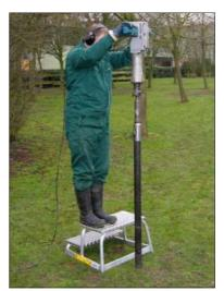
After the first gouge has been inserted into the ground, the striking pen is replaced with an extension rod to assist in pulling it out. Then the rod puller extension (=bottom and top plate and two ABS pipes) is placed over the bar (see drawing). The mechanical rod puller with the casing and rod puller clamp can now be placed on top of this. At this height, the gouge can be pulled out of the ground.
