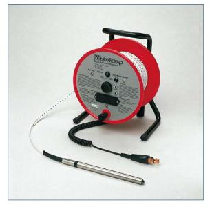
To measure the thickness of a product layer, lower the probe into the well until the signals activate. If there is an oil/product layer on the top of the water (LNAPL), the light and tone will be steady, indicating an air/product interface.
